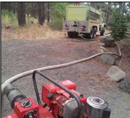
From the Cougar Creek fire: New HPFD tender pumping water from a creek. Photo: Dave Thom
